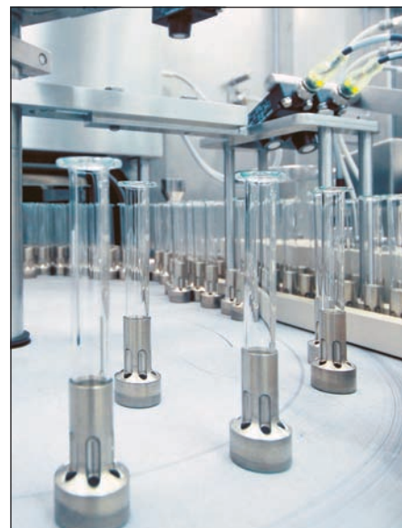
Centocor R&D Schaffhausen: Syringes being transported to the sterilization tunnel.
