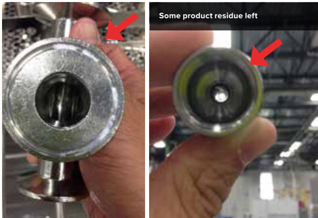
Figure 9: Cream residue on process part after wash cycle
