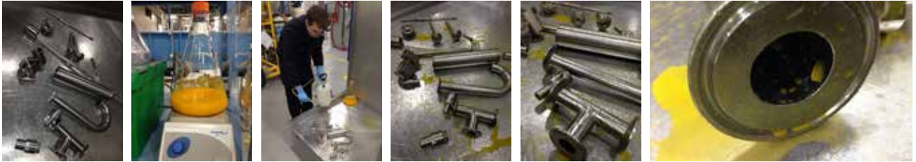
Figure 5: Process parts covered with riboflavin
