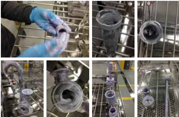
Figure 7: Parts covered with soil
