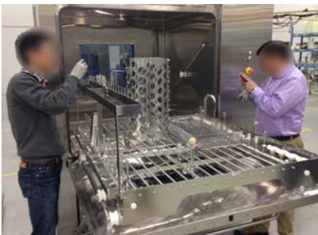
Figure 8: Parts inspection after a wash cycle
