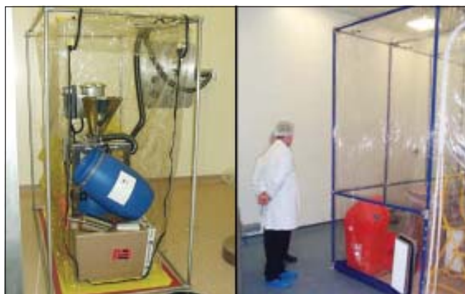
Figure 9. Temporary flexible enclosures: (a) Temporary containment enclosure for Comil (b) Walk in enclosure for active powder campaign.
