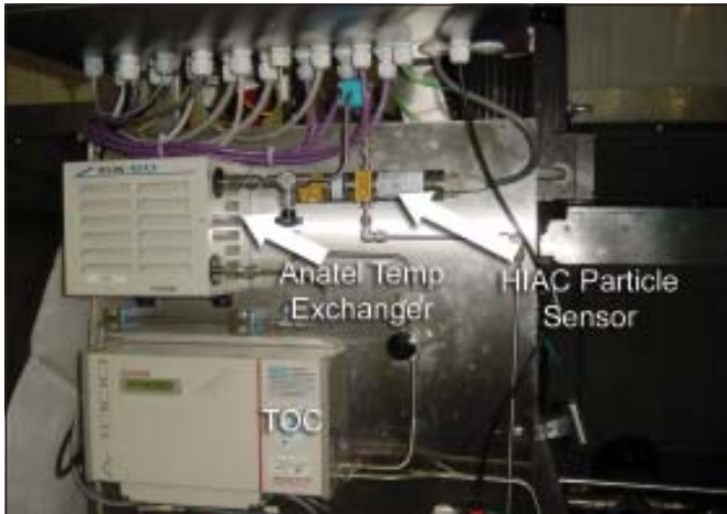
Figure 3. Instrumentation panel with HIAC HRLD sensor.
