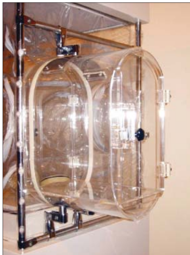
Figure 4. Machined acrylic airlock – easier operation than zipper doors.
